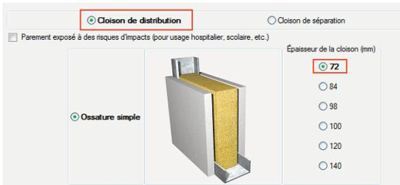
Figure 64 - Cloison de distribution
