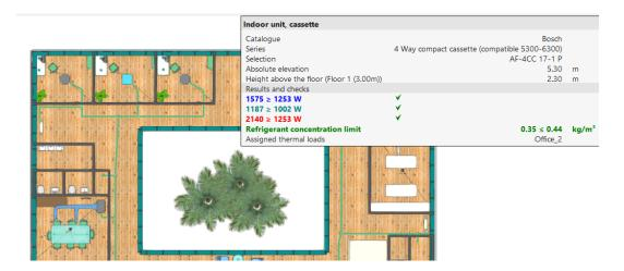
The software also selects the **size** of the **units** according to the thermal loads.
