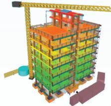
StruBIM Analysis is a tool destined to generate, edit and analyse an analytical model that has been developed based on a structural model (imported using an IFC or XML format file). The analysis of the building demands is carried out by a spatial 3D analysis using stiffness matrices. Users can choose the analysis engine (OpenSees™ or CYPE Frontal Solver).
