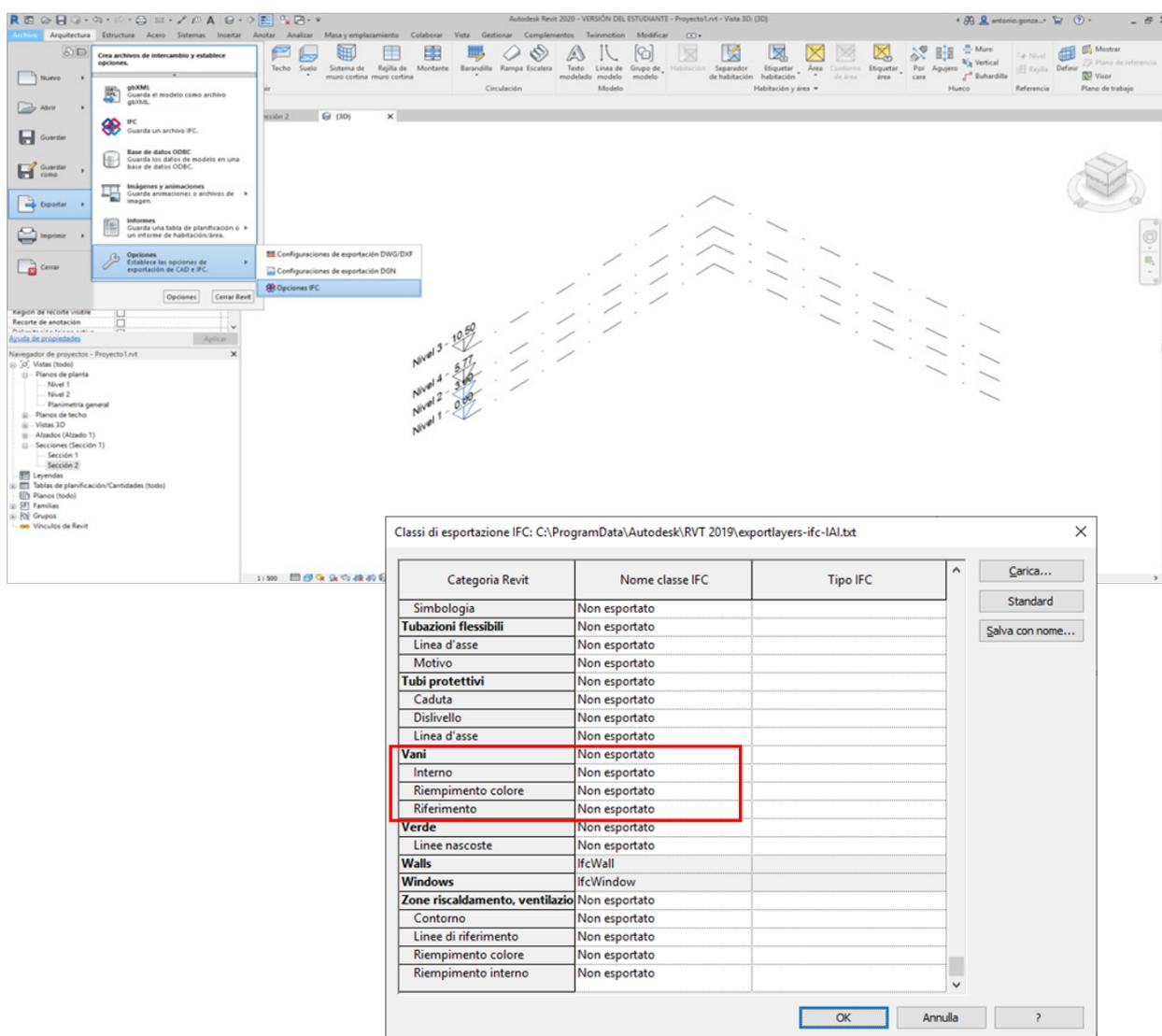
The screenshot shows the Autodesk Revit 2020 interface. The 'Export' menu is open, and the 'Options' sub-menu is selected. The 'Options IFC' dialog is open, showing a table of IFC export classes. The table has three columns: 'Categoria Revit', 'Nome classe IFC', and 'Tipo IFC'. The 'Vani' category is highlighted with a red box.
