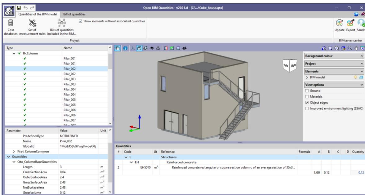
The screenshot displays the Open BIM Quantities software interface. The main window shows a 3D model of a building with a staircase. The interface is divided into several panels:
